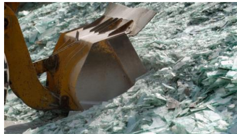
ISOVER, glass recycling 80% of input material for glass wool production in Lucens
